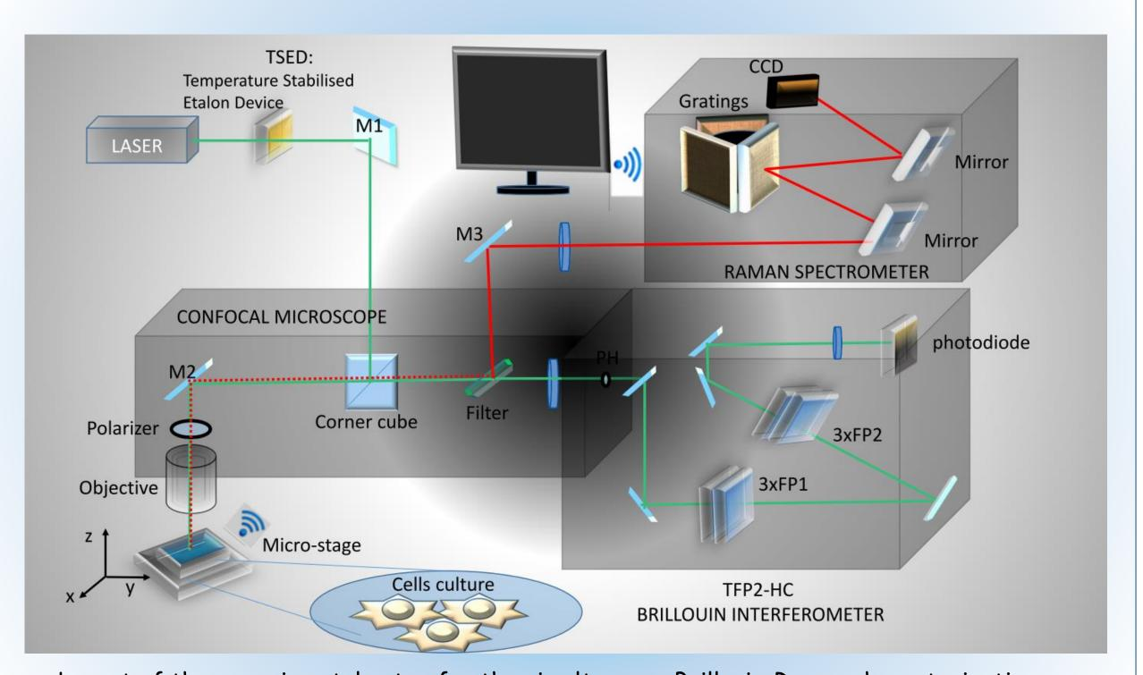
Layout of the experimental setup for the simultaneous Brillouin-Raman characterization.
