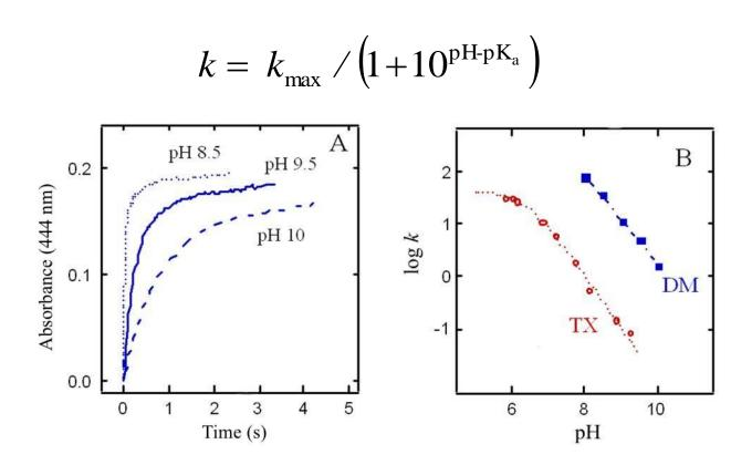
ET to the catalytic site is regulated by the protolytic group with  $pK_a$ =6.6
