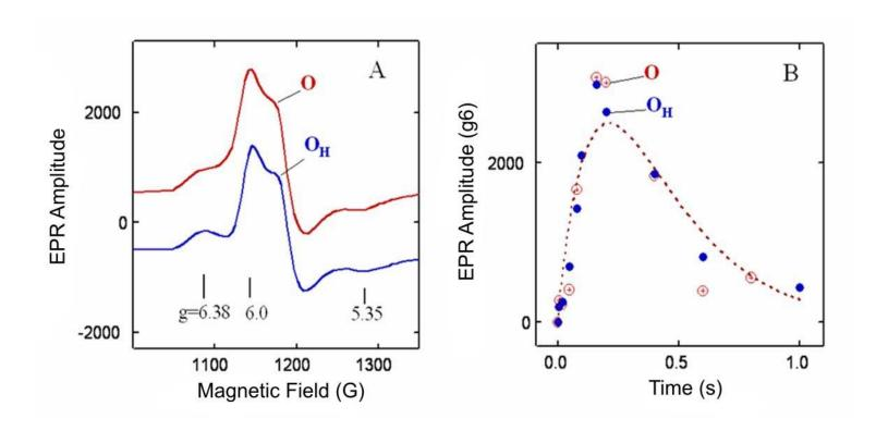
Spectral (EPR+ UV-VIS absorption) and kinetic equivalence of O and  $O_H$  forms of oxidized CcO
